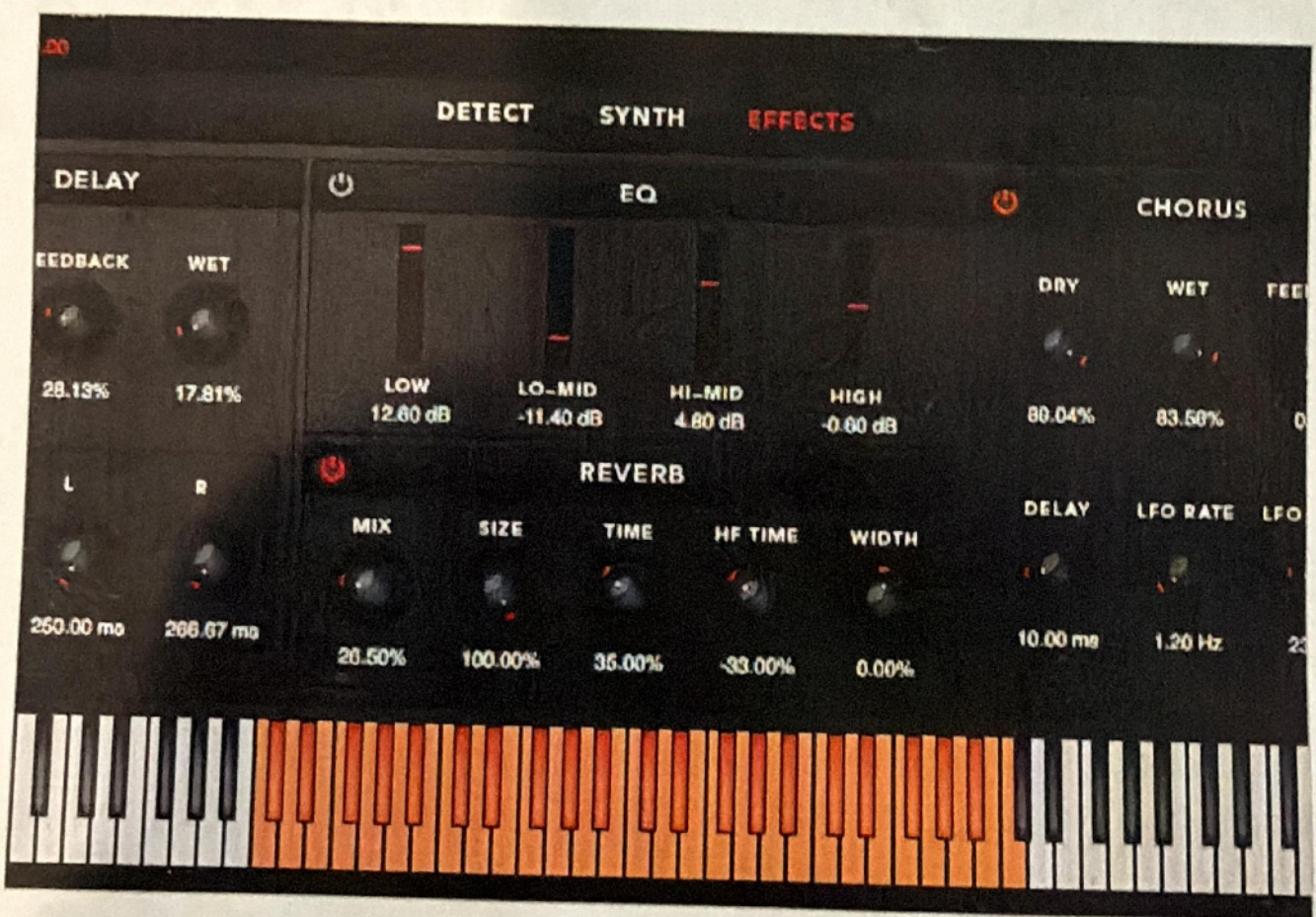
Fig. 23: A graphic EQ gets its name because the sliders draw a “graph” of the frequency response.
