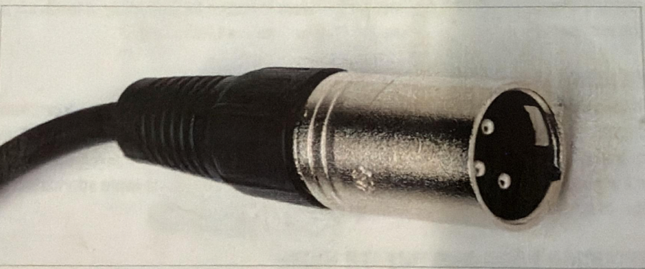
Fig. 7: An XLR plug, as used for balanced line connections.
