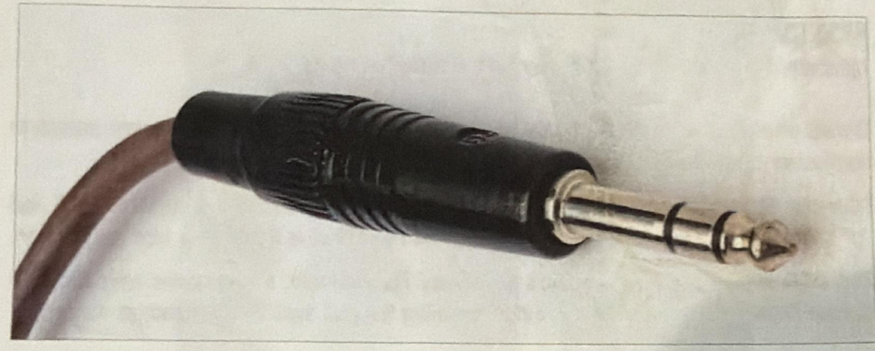
Fig. 6: A balanced (TRS) 1/4" phone plug. Note there are three sections, separated by black insulating bands—the tip, the ring, and the ground. These are also called stereo plugs when used to carry two independent left and right channel signals.
